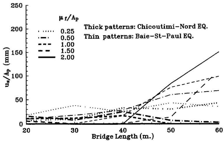
Figure 5 Transverse sliding displacement per peak ground acceleration (%g) of 2-lane bridges for various friction coefficient to PGA ratio (Eastern Canada earthquakes)
