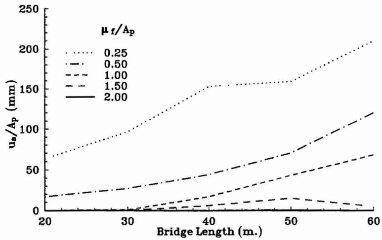
Figure 3 Transverse sliding displacement per peak ground acceleration (%g) of 2-lane bridges for various friction coefficient to PGA ratio (average of Western USA earthquakes)
