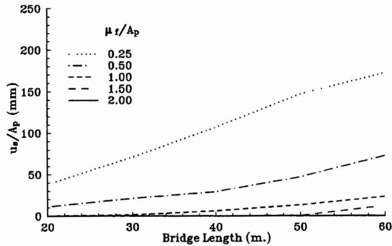
Figure 4 Transverse sliding displacement per peak ground acceleration (%g) of 3-lane bridges for various friction coefficient to PGA ratio (average of Western USA earthquakes)
