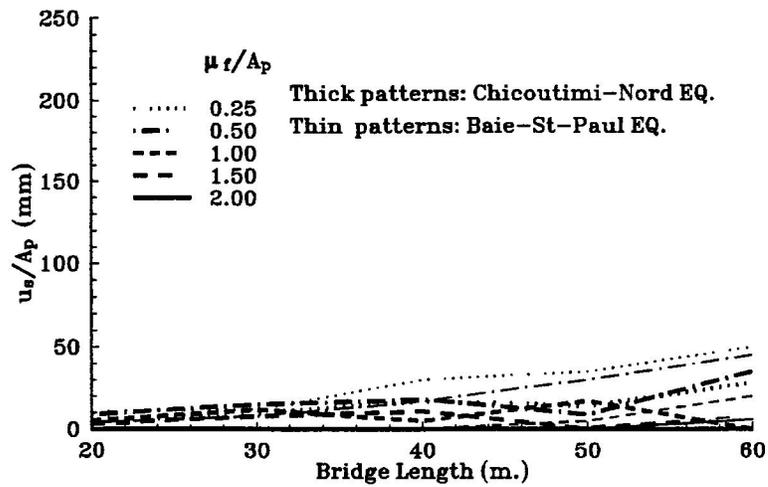
Figure 6 Transverse sliding displacement per peak ground acceleration (%g) of 3-lane bridges for various friction coefficient to PGA ratio (Eastern Canada earthquakes)
