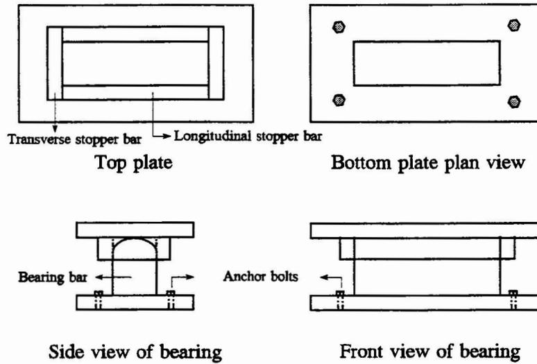
Figure 2 Typical fixed sliding bearing
