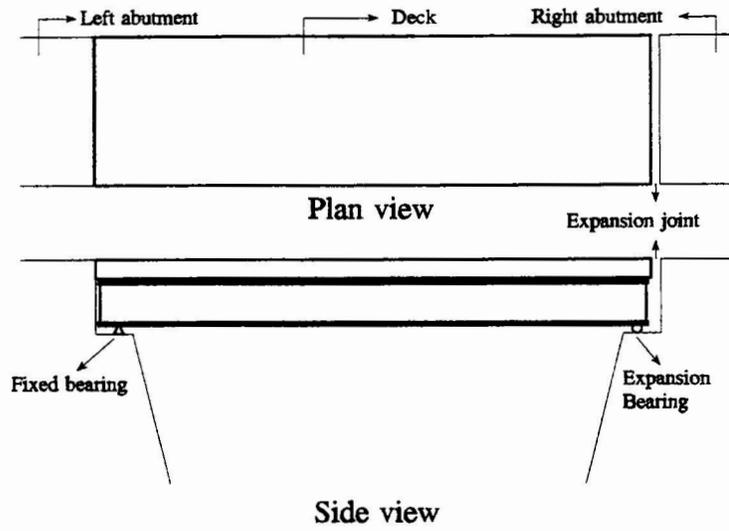
Figure 1 Typical single-span simply supported bridge
